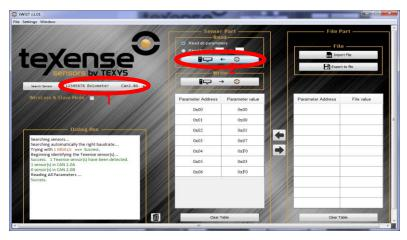
Change the parameters according to its specification sheet and click on the write button to send the parameters to the sensor. You can read it back to ensure the modification was acknowledged by the sensor. Any out-of-bounds writing will be replaced by the default value.
