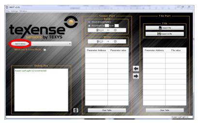
Once the search is done the list next to the search button should contain all the texense sensors detected on the CAN bus (1). Select the sensor you want to configure and click on the button in the read panel (2) to display sensor's configuration:
