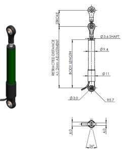
**ELPM-SO version with spring loaded shaft**
