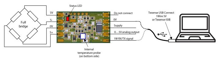
Note: it is also possible to build half bridge and quarter bridge versions by adding resistors. Please refer to XN4 operating manual for complete information.
