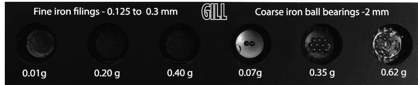
Debris Strip (Part No. 4212-00-063)
